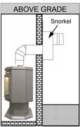
**IMPORTANT:** Do not locate termination head where excessive snow or ice build up may occur. Check termination head area after every snow fall, and clear if necessary to prevent blockage. If using snow blowers, make sure snow is not directed at the termination head.
